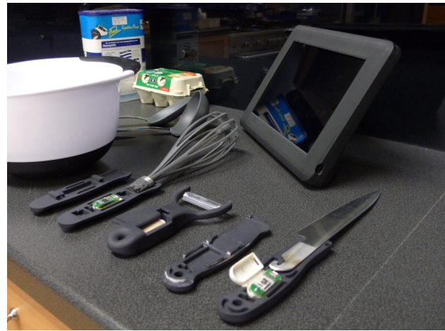
Figure 2: Some of the 27 kitchen items instrumented with accelerometers
